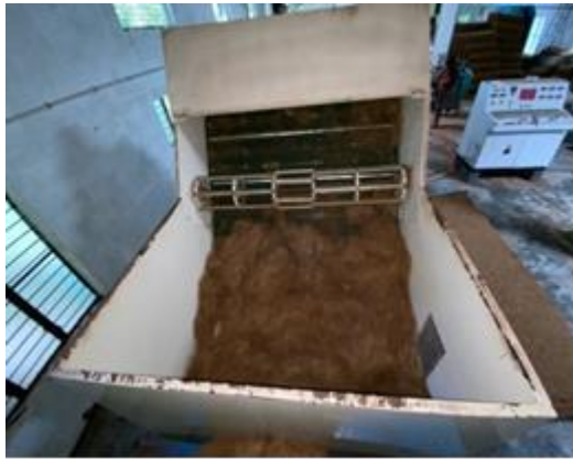
Figure 1: Laying of the Coir fibres
