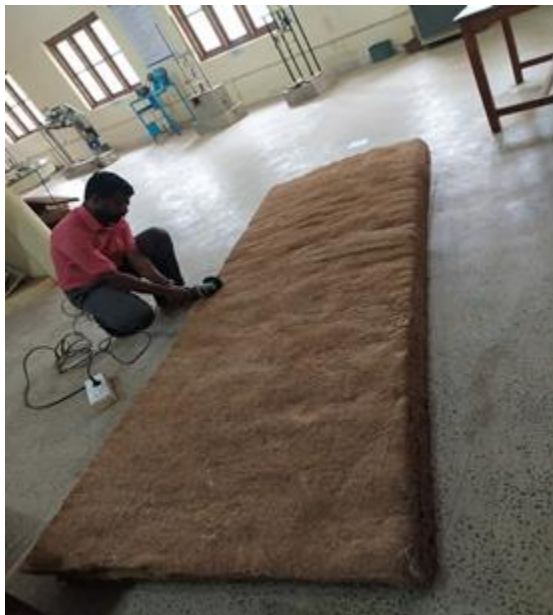
Figure 3: Developed Needle felt Coir-Latex Composite (NFCLC50)
