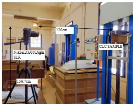
Figure 4: Typical experimental setup for the Poisson's ratio test
